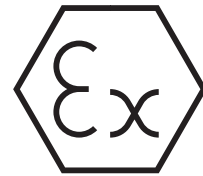
Fig. 0 A - Specific marking for protection against explosions - Directive 94/9/EC.
